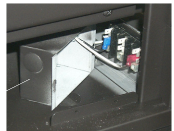
Remove cover to access Terminal Block
