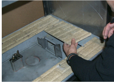
Remove Left & Right Side Base Brick Panels
