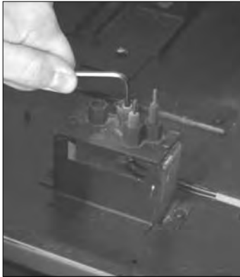
Figure 53: Removing the Pilot Orifice.
