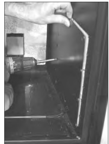
Figure 57: Removing Access Cover.
