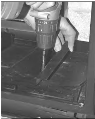
Figure 56: Removing the Right Burner Support.
