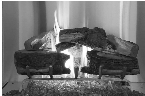
Figure 8 - Correct Burner Flame Pattern
