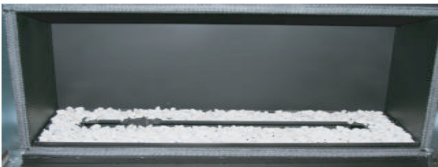
Figure 39 - Filling the tray with media
