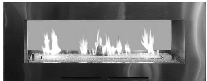
Figure 9 - Incorrect Burner Flame Pattern caused by port blockage
