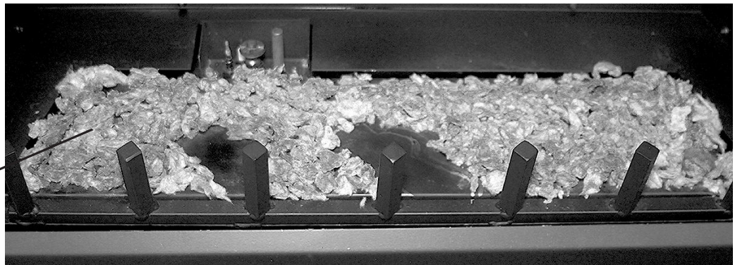
Figure 16 - Rock Wool Placement
