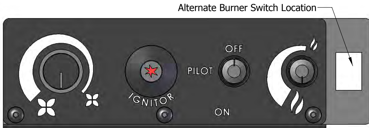
Figure 6: E20 Control Panel.
