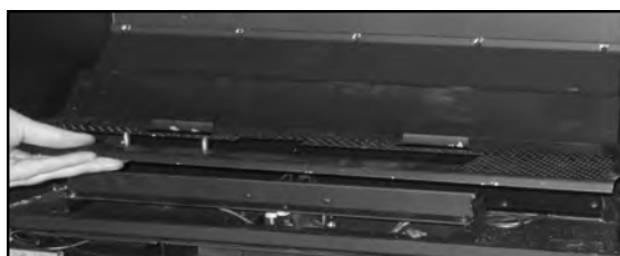
Figure 55: Burner Tray Installation.
