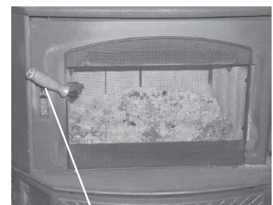
Handle at 10 o'clock position.
