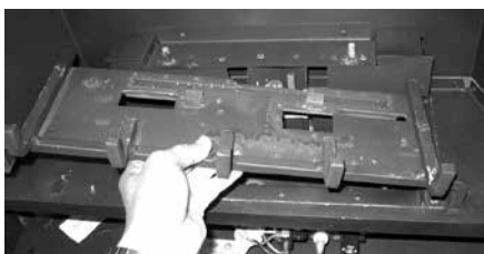
Remove the 2 screws, push Burner Assembly to the left and lift out.
