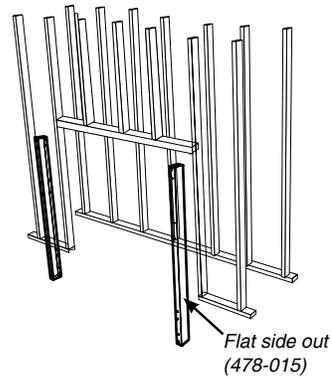
5. Secure horizontal steel header with 2 screws per diagram
