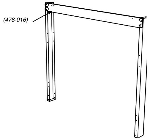
6. Slide the unit in position. Hook up gas, venting and electrical and fan (if purchased) prior to installing the remaining horizontal steel studs.
