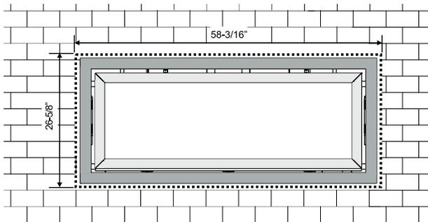
For material such as brick, stone, etc that extends 3-1/8" or less , the minimum opening dimensions noted below must be adhered to when finishing around the unit. This is to ensure the removal of the faceplate and for the safe operation of this appliance.
