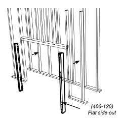
Secure horizontal steel header stud (466-128) with 2 screws per side as per diagram.
