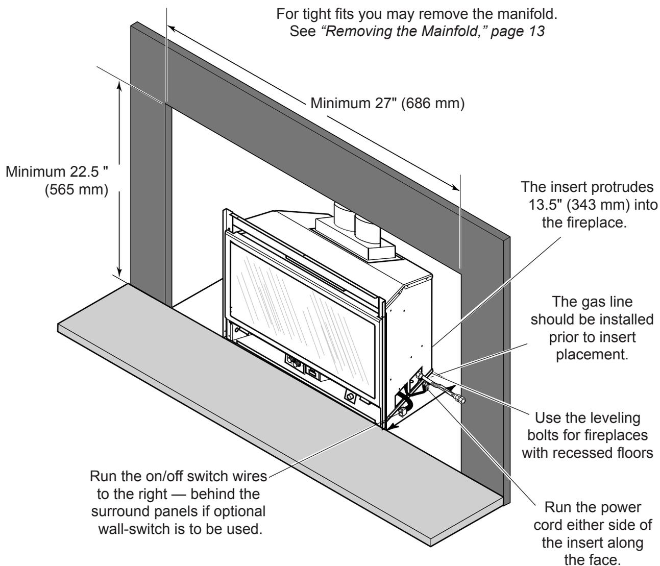
**Figure 3 - Insert Placement**
