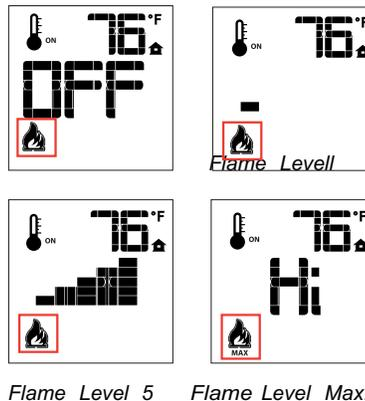
Figure 21 - Remote Control Displaying Flame Levels
