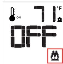
Figure 21b - Remote Control Displaying Split Flow Mode
