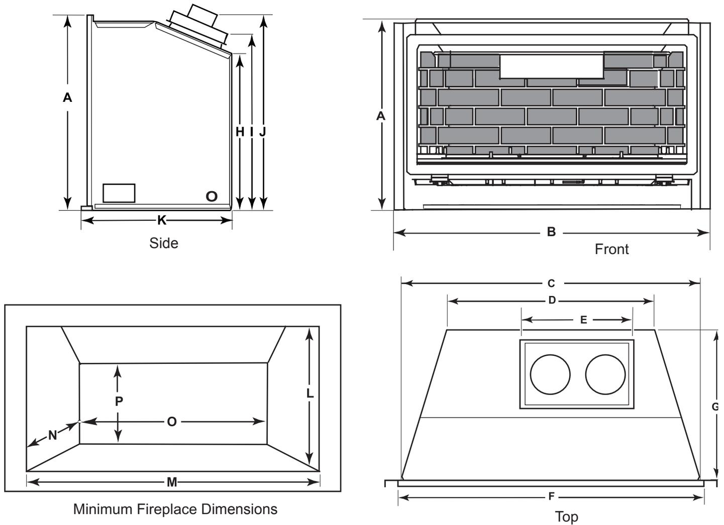
**Figure 2 - Minimum Fireplace and Insert Dimensions**
