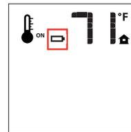
Figure 24a - Remote Control Displaying Low Battery
