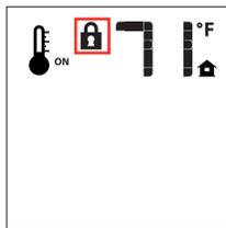
Figure 34 - Remote Control Displaying Key Lock Mode
