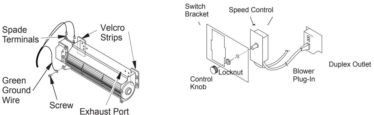
**NOTE:** Unplug powercord before servicing. The blower is attached to the insert bottom and back with Velcro. To remove blower for servicing, pull away from Velcro and disconnect wires.
