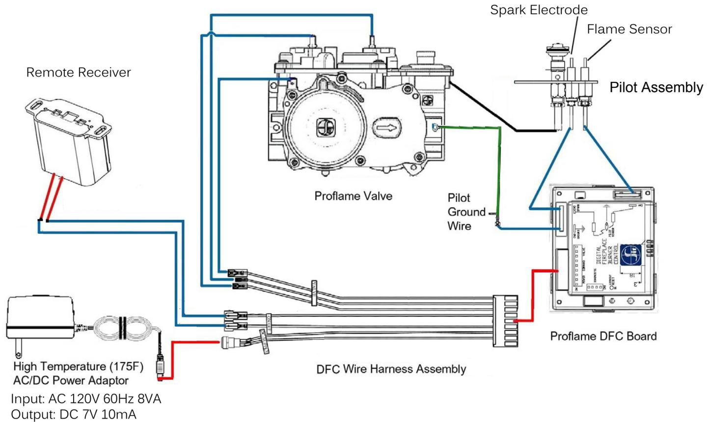
\*) The Remote Control Receiver is a standard feature for this appliance. If Wall Thermostat or ON/OFF switch are required for operating, replace the Remote Receiver with desired device using existing wires. Clear contacts (mV rated) to be used. **Do not connect to 110V !**
